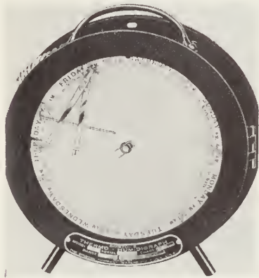
22-8. A seven day recorder for both the temperature and humidity. These records are important as a means of checking on the efficiency of the air conditioning system. (The Bristol Co.)
